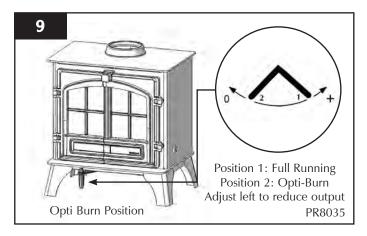
• Lowest heat out put for burning wood (Opti Burn). This position helps keep the glass clean, Diagram 9
